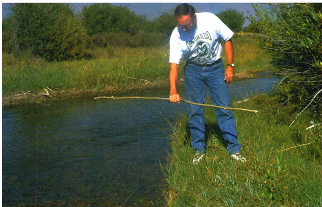
Figure 16 —Correct placement of the sampling pole along the greenline water interface.
