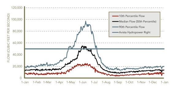
Figure 15: Hydrograph of Clark Fork River at Noxon with Avista hydroelectric water right
