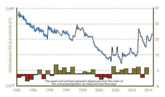
Figure 19: Groundwater levels in a well near Roundup showing the effect of the 2000s drought
