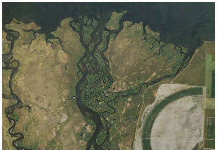
Braided D channel classification on the Madison River above Ennis Lake due to the influence of the sediment deposited on the delta.
