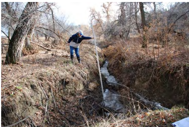
Channel is deeply incised, active downcutting. No riparian area present. Stage 2 Schumm's Model = Score 0.
