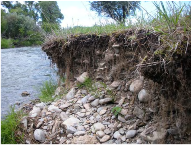
The fine roots of quackgrass and smooth brome may be deep as seen here in this unconsolidated gravel and cobble material, but they don't have the mass and strength to provide the necessary bank stability.
