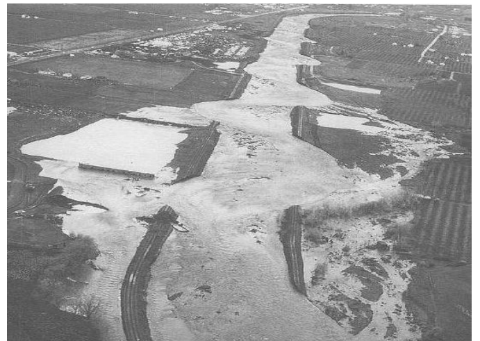
Sediment transport function is regulated by channel dimension, gradient, and discharge. Channel modifications that don't recognize these relationships are doomed to fail. Walla Walla River 1964 (OSU Archives).
