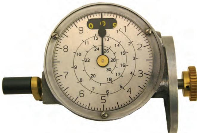
**Figure 57.** Computing depth indicator.
