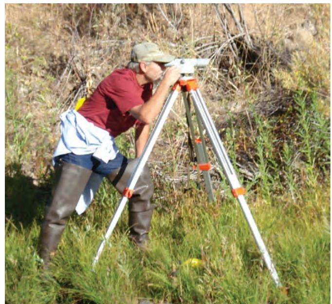
Figure 7. Surveying level and tripod.
