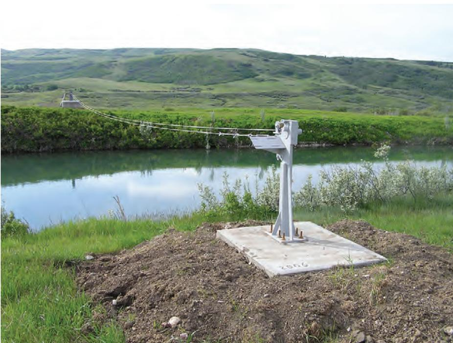
**Figure 65.** Bank-operated cableway.
