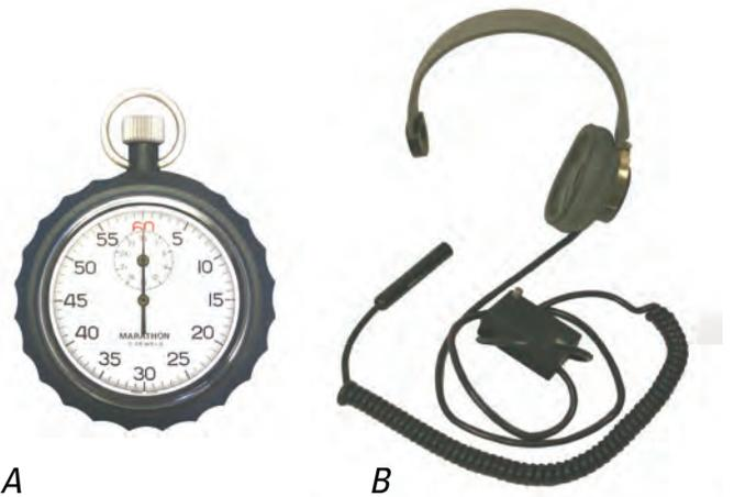
**Figure 33.** A, Analog stopwatch and B, current-meter headset.
