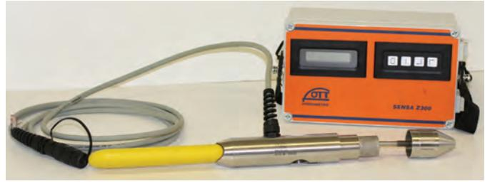
**Figure 39.** Ott electromagnetic current meter.
