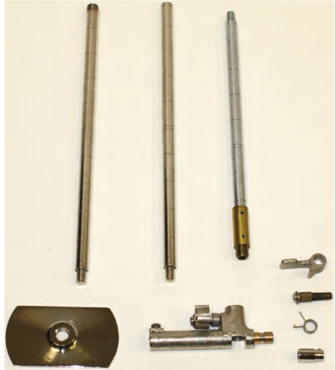
**Figure 47.** Parts for the round wading rod.
