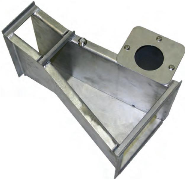
Figure 77. Modified 3-inch Parshall flume.
