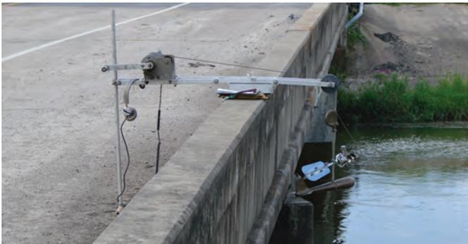
**Figure 66.** Measuring from a bridge with a bridge board.
