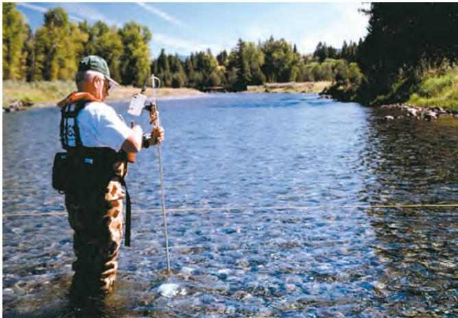
**Figure 17.** Wading measurement using a top-setting rod.
