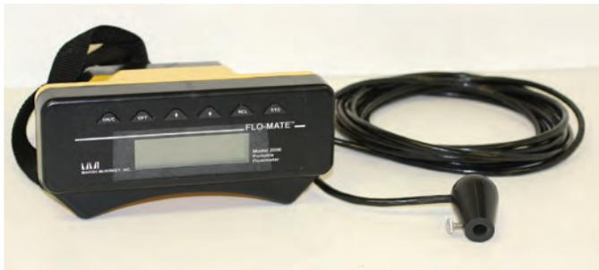
**Figure 38.** Marsh-McBirney Model 2000 electromagnetic flowmeter and display meter.
